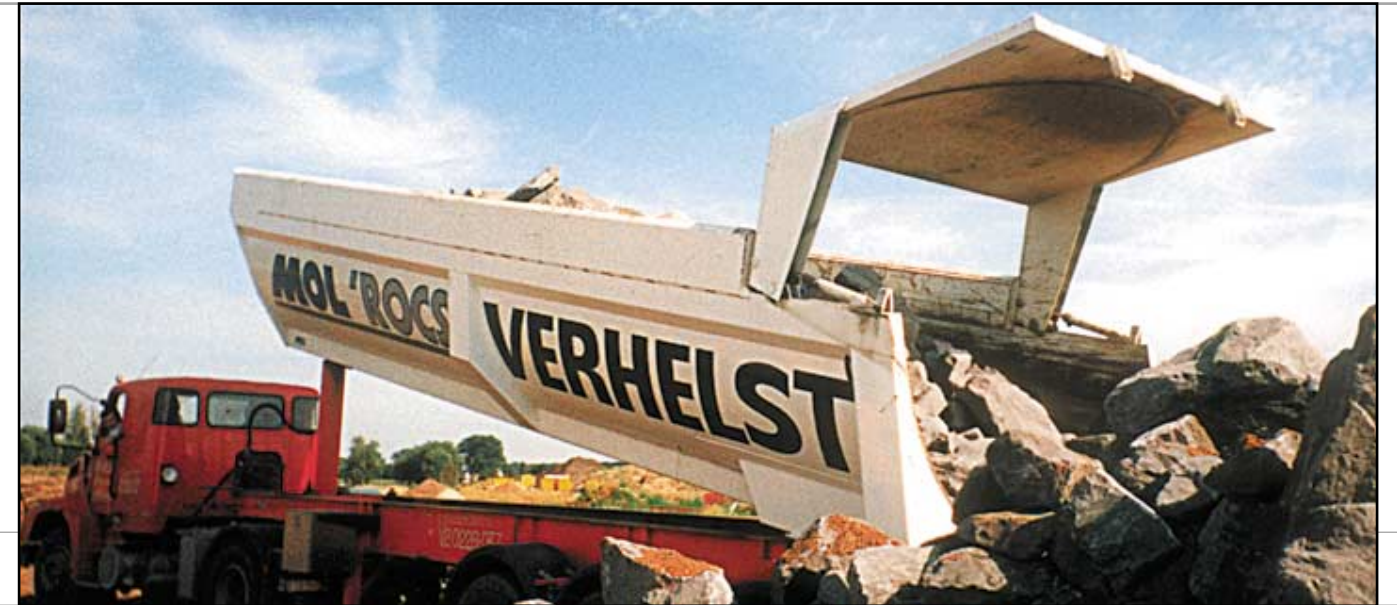
tippers for quarry stone up to 6000 kg a piece
